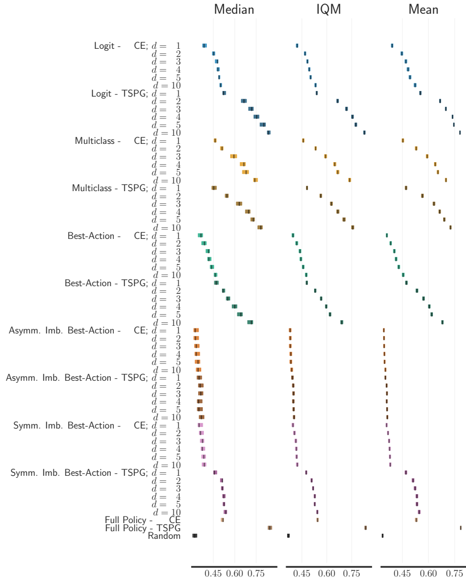
Figure 11: Aggregate metrics for the performance levels of all 63 agents in the set of thirty games. Median, interquartile mean (IQM), and mean of the win rates are computed over runs in all games against all possible opponents. Coloured bars represent 95% bootstrap confidence intervals, estimated from 10,000 bootstrap replicates using the rliable library [67].
